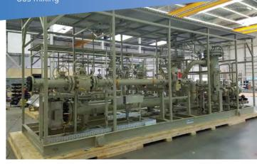
The standard gas filter units are usually designed according ASME B31.3 and ASME VIII div. 1 and can be supplied with, but are not limited to, the following certification;
