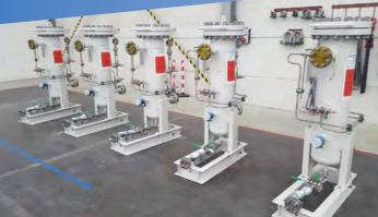
All standard configurations are available in carbon steel, low temperature steel and stainless steel for both the filter housing and piping. Standard connection sizes are 1" to 8" and pressure rating from 150# to 900#.
